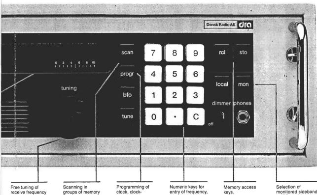
Free tuning of receive frequency in 1000, 100 or 10 Hz steps and manual scanning also reverse.
